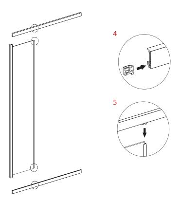
Step 4 - Install the guide rail covers by sliding these into and along to the end of the recess in the top and bottom frame extrusions.
