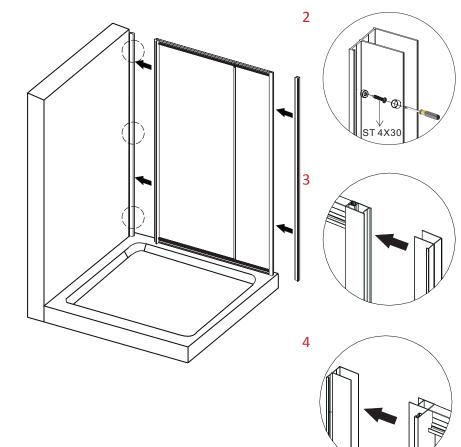
Step 2 - Working from the INSIDE of the shower install screws / cap retaining collars through wall receivers and into the wall anchors or wall. Run a small "eyebrow" bead of silicone onto the thread as you insert the screw.
