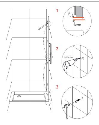
Step 1 - Measure and mark on the wall surface 10mm INSIDE of the outer edge of the tray. Repeat on the other side of the tray.
