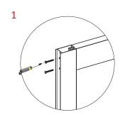
Step 1 - Fasten the fixed glass panel to the top and bottom frame extrusions with 4 x 3.5x30mm frame fixing screws.
